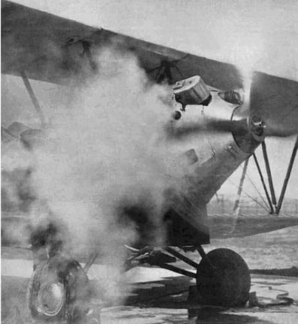
A Travel Air 2000 biplane made the world's first piloted flight under steam power over Oakland, California, on 12 April 1933. The strangest feature of the flight was its relative silence; spectators on the ground could hear the pilot when he called to them from mid-air.
